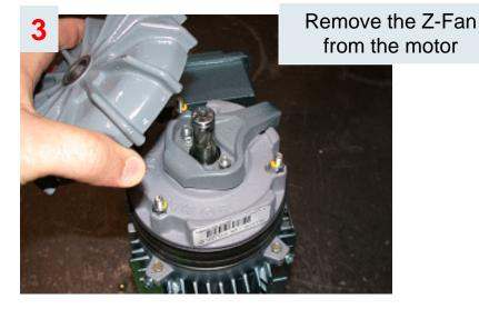
With the medium sized flat-tip screwdriver, gently pry the fan up and down to loosen and remove it. Use caution to avoid damaging the fan!
