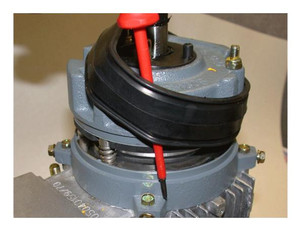
• Re-install the 2 brake band clamps using the flat tip screwdriver.
