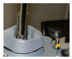
Verify the free play on the release arm. adjust the locking nuts as needed to achieve 1.5 – 2.0 mm gap. (S Dimension)
