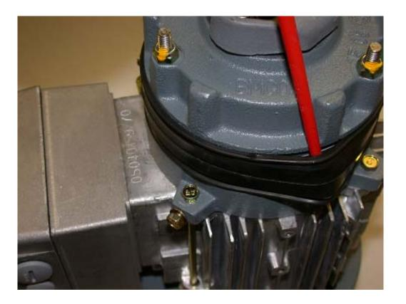
Using the metric feeler gauge, determine the current air-gap setting.
