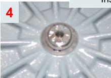
Re-install the snapring using the snapring pliers.
