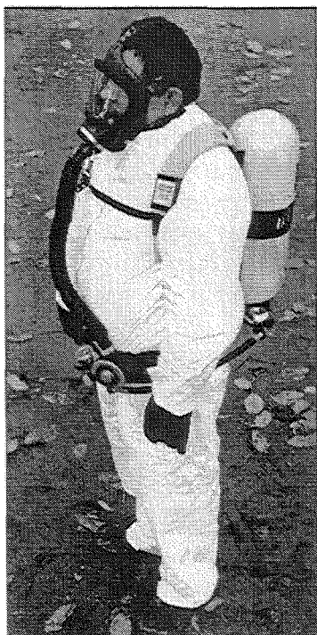
Figure 6-12. A self-contained supplied air respirator provides uncontaminated air from a compressed air tank.
