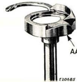
Fig. 22. Sewing Hook Removed from Machine Showing Hook Washer
