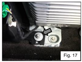
31. Remove the bolt (this bolt will be re-used), factory subwoofer stud and two screws (these two screws will be re-used) securing the factory amplifier bracket. You will also need to release the retainers securing the factory amplifier harness to the factory amplifier bracket. Remove the factory amplifier/bracket assembly. Fig. 18-19
