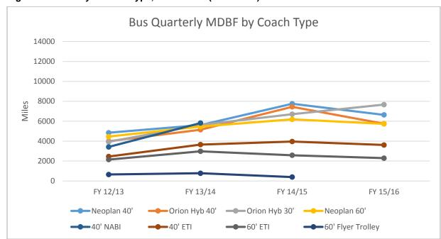
Figure 2: MDBF by Vehicle Type, Older Fleet (2000-2007)
