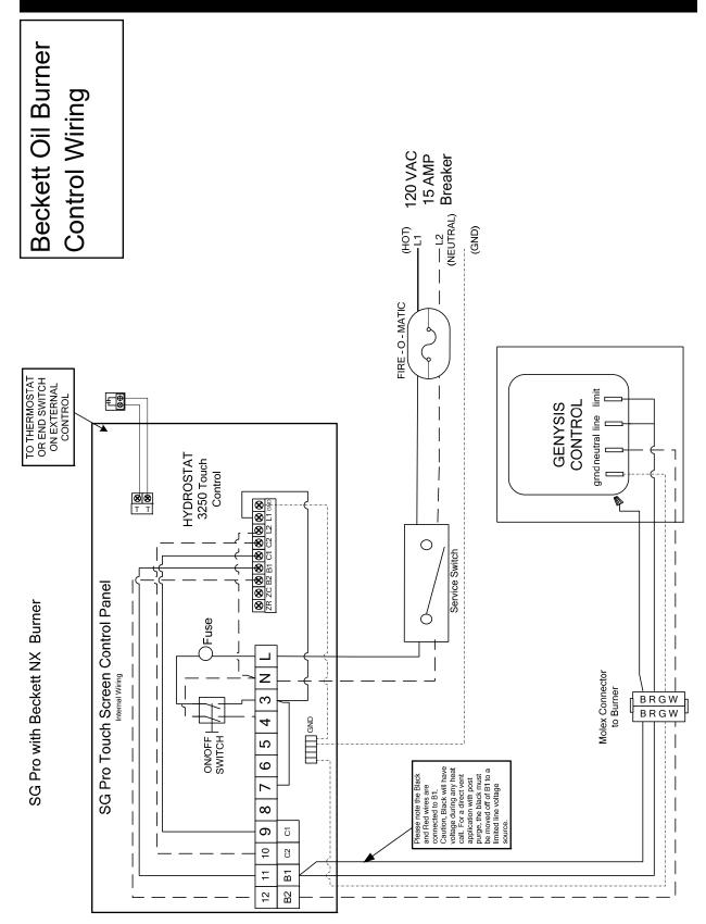
NOTE: All wiring must be done in accordance with applicable state, local and national codes. Use only copper conductors.
