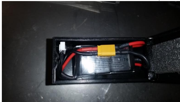
Proper positioning of the battery after connection
