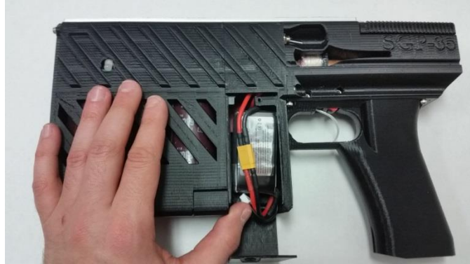
Proper positioning of the battery after connection
