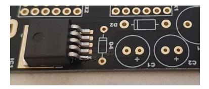
Now you can solder the remaining 4 pads of the IC. Do not solder the tab of the PCB.
