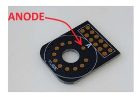
Now you can insert and solder in the tube. Pay attention that the tube sits squarely on the PCB. Then solder on the connector. Keep the tube 5mm (0.2") from the PCB. Failure to keep this separation will invalidate any tube warranty claim.
