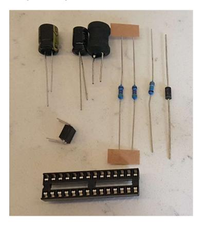
Take care that the notched end of the IC socket is at the end shown. However, if you find you soldered it with the wrong orientation, do not try to remove it. It is perfectly fine with the notch at the wrong end, just be sure to place the IC in the socket with the IC's notch in the correct position.
