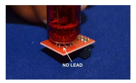
Insert from the side of the PCB with no markings. Pay attention that the tube sits squarely on the PCB. Then solder on the connector.
