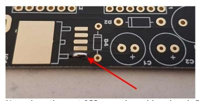
Now place the part IC2 over the soldered pad. Ensure the part is
