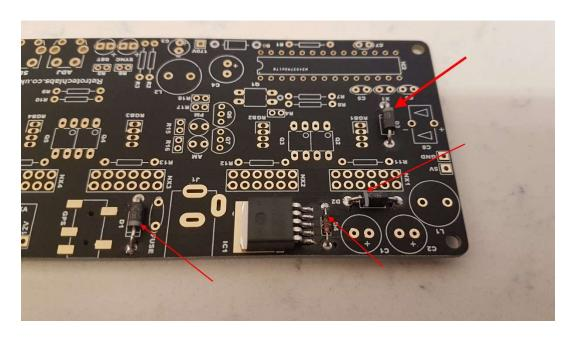
Continue to mount C1, C2, L1, J1 and FUSE. C1 and C2 are polarized. The longer lead goes in the hole marked `+'.
