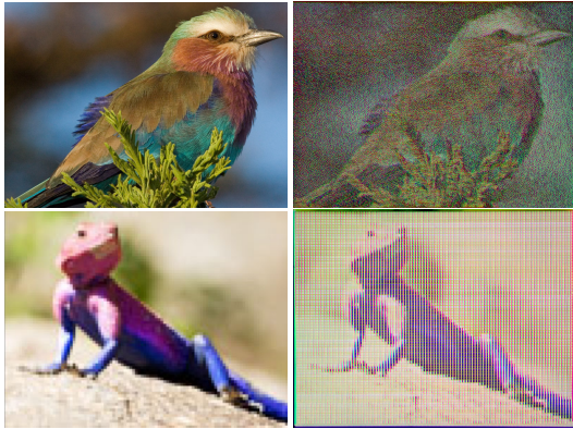
Figure 13: Top Left: An input photograph of a bird. Top Right: A white SHADOWPIX that encodes the red, green, and blue channels of the input as separate images, illuminated by colored lights from three directions, using the global method. Bottom Left: A lower res input photograph of a lizard. Lower Right: A white SHADOWPIX that encodes the RGB channels, using the local method. These images were obtained by capturing three photographs in raw mode, each with a single color light, and adding them in software.
