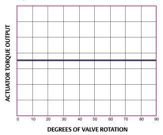
Torque output of the rotary vane actuator remains constant throughout the full rotation of the valve. This ensures that your specified safety factor will not be jeopardized at different positions during the valve stroke. Constant torque output is an especially important feature in the following applications:
