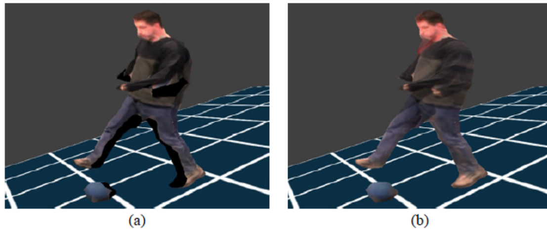
Fig. 7. Two view-dependently textured views of the same visual hull model. The left rendering uses conservative visibility computed in real-time by our algorithm. The right view ignores visibility and blends the textures more smoothly but with potentially more errors.
