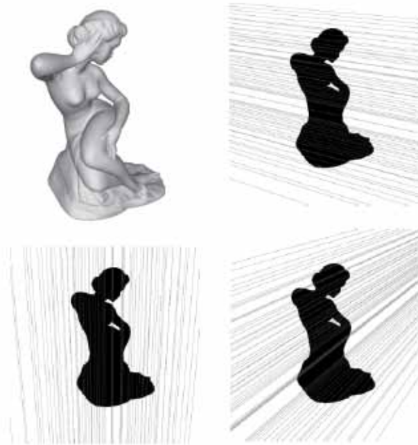
Figure 6: One object (top left) and its silhouette with 2D lines traced over it to find intersections along rays in the X , Y and Z ray-set of the MI, respectively. The number of lines has been reduced for illustration purposes: in typical cases they would cover most of the area of the image.
