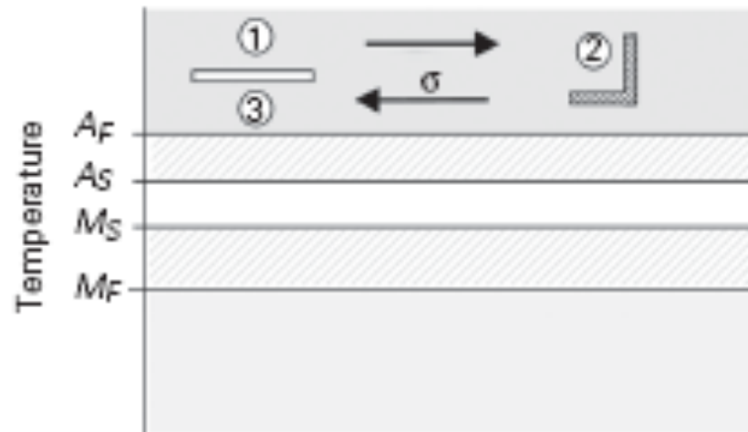
Figure 1. Pseudoelasticity. A_S , A_F and M_S and M_F = temperature at which the formation of austenite and martensite starts and ends, respectively. \sigma - \epsilon = stress-strain curve. See text
