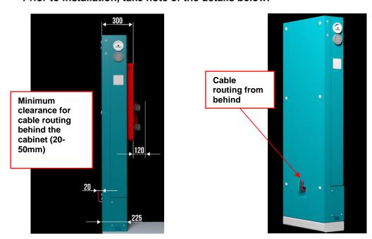
Note that the Cabinet need to swing open for service, so the area seen below must not have obstacles higher than 350mm. A free area of 30mm above the top of cabinet is needed when doing service.
