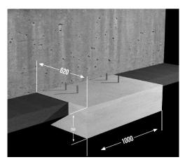
Drill hole for 4 psc of Expansion-anchors and fit according to instruction.
