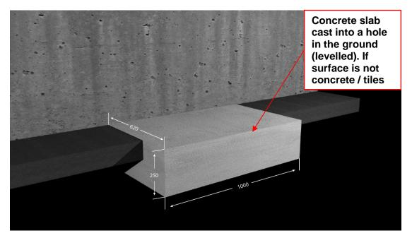
Size of Concrete Slab (plate) need to be at least **Width**=1.0m x **Length**=0.5m.
