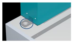
After the Sharebox Auto S18 is properly fixed to the conrete slab. The front plate and top-plate can be put back on and fixed with the torx screws used for removing it.
