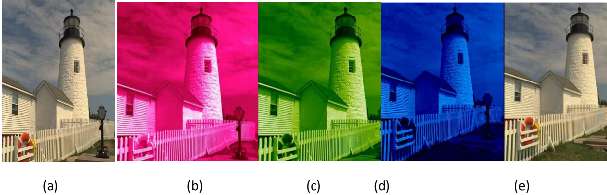
Fig 5: (a) Original Light House Image (b) Red Channel of Light House Image (c) Green Channel of Light House Image (d) Blue Channel of Light House Image (e) Demosaicked Light House Image.
