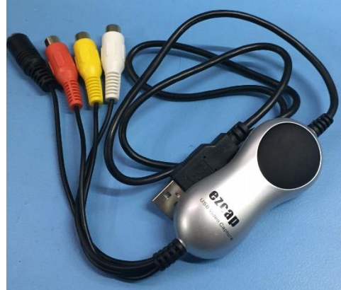
USB2 video frame capture device. Shows in SharpCap as a USB 2861 device .
