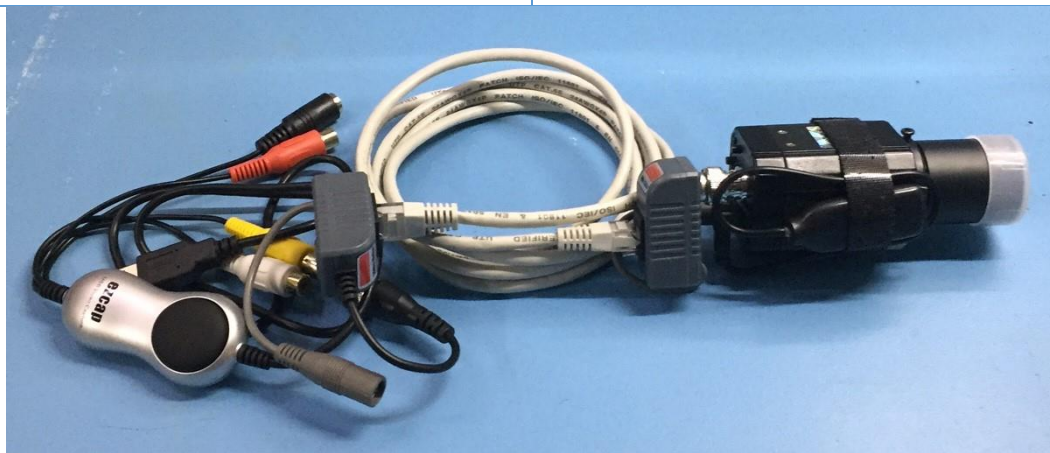
From left to right – video frame grabber, balun, ethernet cable, balun, analogue video camera.
