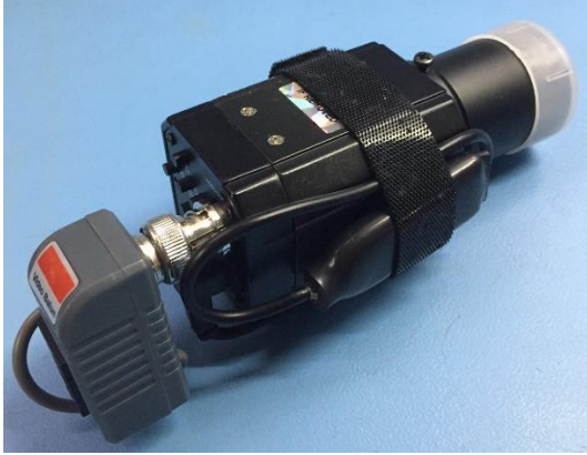
Analogue video camera with Bluetooth adapter for accessing the camera's internal menu. Video/power balun (left hand side) used to connect ethernet cable.
