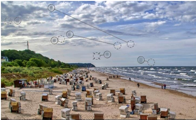
The sensor spot corrector marks all of the patches and determines a source within the image that can be used as a substitute.
