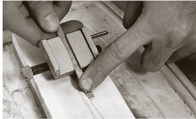
WHEN HONING NARROW TOOLS, THIS is the best way I’ve found to keep things steady and square. Put one finger on the cutting edge; put the other behind the jig to move it.
