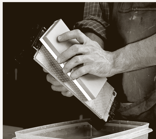
NORTON WATERSTONES AND THE DMT DuoSharp stone are a great combination. The DMT handles the grinding jobs and flattens the Norton waterstones.
