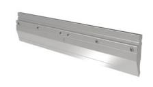
Upper adapters have very precise dimensions and limited height. They are studied to be mounted directly to press brake upper beam and when mounted, they can host punches with a different tang than the original one. Such solution is very interesting when you have to retrofit a press brake: in a press brake with a special tang you can mount all standard tools in the catalogue.
