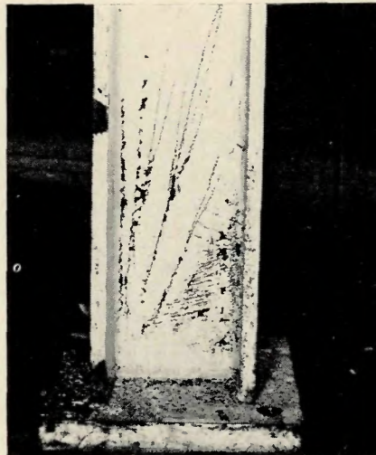
Fig. 21—Plastic region above base plate ( V = 216 kips)
