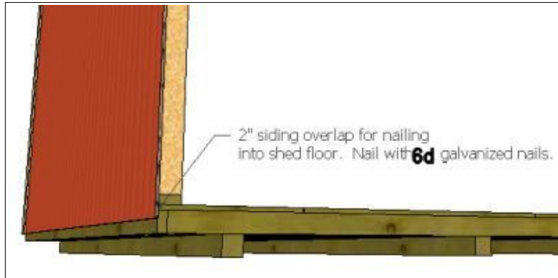
Extend Siding Below Floor Sheeting
