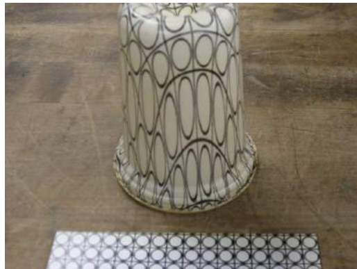
Figure 15-8 Strips of varying width are stretched to obtain different e_2/e_1 ratios.
