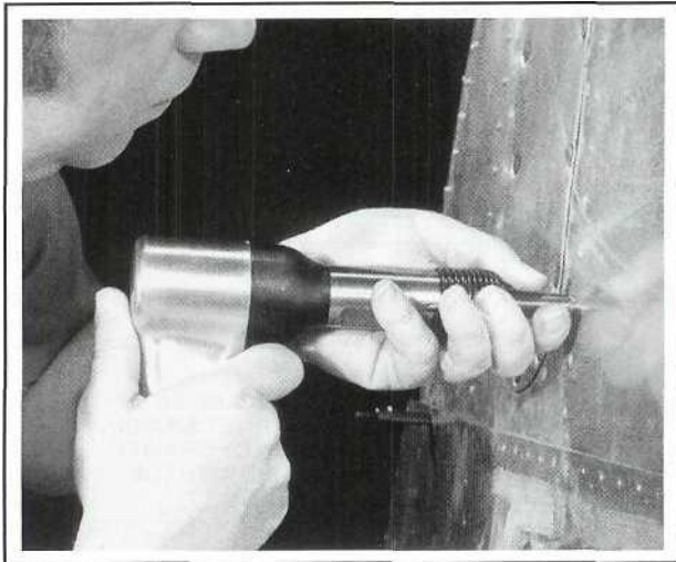
Figure 2-120. Hold the rivet set square with the rivet head and support the gun so the set will not slip off during driving.
