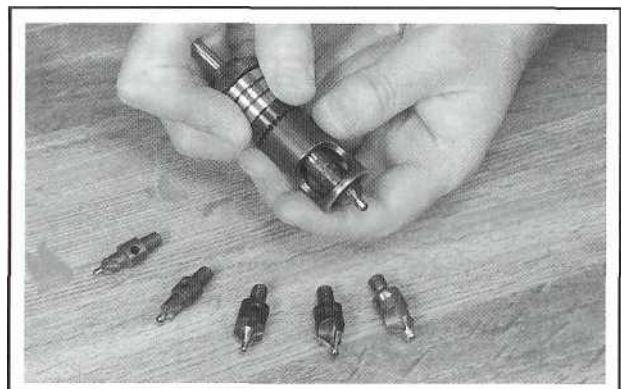
Figure 2-106. Countersink cutters and the cutters used in micro-stops are manufactured with a 100 degree cutting angle. With some cutters, a pilot is milled onto the end while others have interchangeable pilots. Pilots are available in various sizes to match the diameter of the rivet shank and help position the cutter in the center of the hole.
