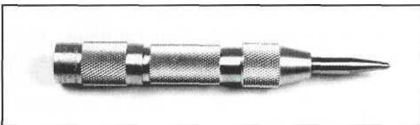
Figure 2-23. An automatic center punch makes uniform indentations for aligning tools such as drills and hole cutters.
