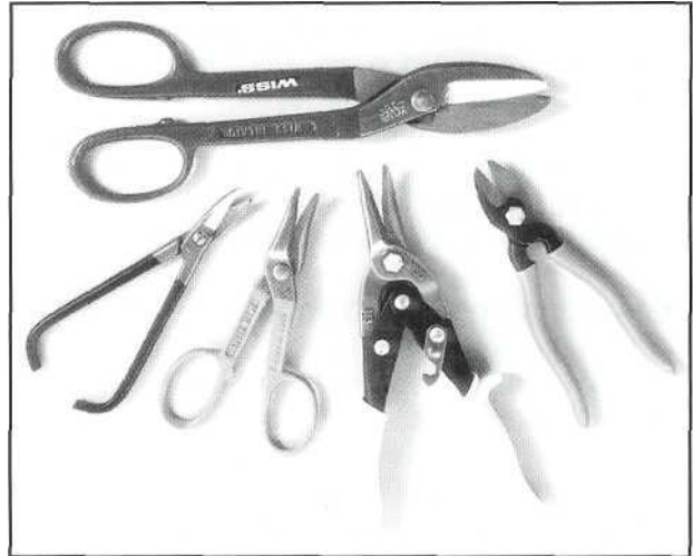
Figure 2-29. Hand shears and aviation snips are used for cutting thin sheet metal.
