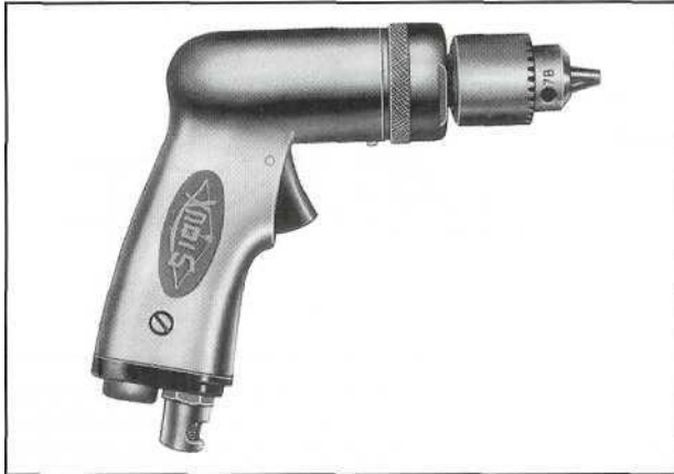
Figure 2-39. A pneumatic, or air drill motor, is the most widely used drilling tool for aircraft sheet metal repair work.
