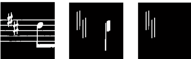
Fig. 4. Shows the process of identifying sharps in a key signature. The original image (left) is eroded and then dilated with a vertical line (middle) and then extra filters based on the shape are applied (right).
