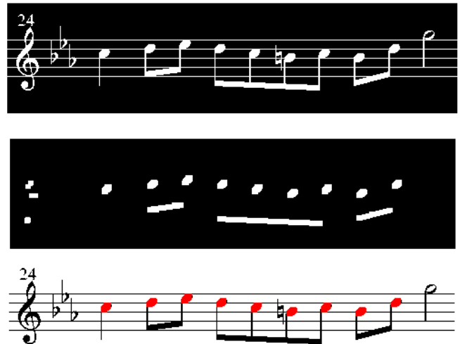
Fig. 5. Shows the process of detecting quarter and eighth notes. The original image (top) is eroded and then dilated with a small disk (middle) and then the connected components are thresholded by eccentricity and area (bottom).
