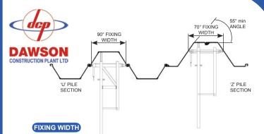
The 'Fixing Width' is the distance between Hard Point tips when installed on any given sheet pile(s). Each Redeb model has a minimum achievable and maximum allowable fixing width' and this is different in both cases depending on whether 70° or 90° Hard Points are used. The maximum allowable fixing width must not be exceeded as this will lead to bracket damage and possible system collapse.
