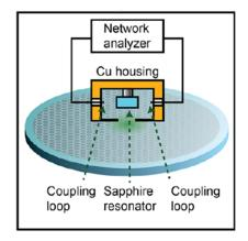
**Figure 2.** Schematic of a scanning dielectric resonator system in which the dielectric resonator is housed in a conducting box, with an aperture through which the fringing field extends (see [13]).
