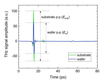
**Figure 3.** Time-domain traces through a bare substrate glass wafer and through a coated wafer, showing reduced transmission through the coated wafer and indicating the peak-to-peak values used in calculating frequency-averaged sheet resistance.
