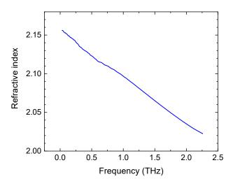
**Figure 5.** Refractive index of the substrate glass wafer measured by THz TDS; used in calculations of sheet resistance.
