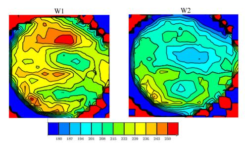
**Figure 7.** Sheet resistance contour maps for two 200 mm diameter wafers. W1: Mean value 223.2  $\Omega$ , standard deviation  $\pm$  19.9  $\Omega$ . W2: Mean value 202.1  $\Omega$ , standard deviation  $\pm$ 15.1  $\Omega$ .
