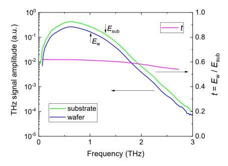
**Figure 4.** Spectra of THz beams transmitted through a bare substrate glass wafer and through a coated wafer, calculated from time-domain data in Figure 3, showing reduced transmission through the coated wafer. The red line (right-hand axis) shows the transmission ratio used to calculate frequency-resolved sheet resistance.
