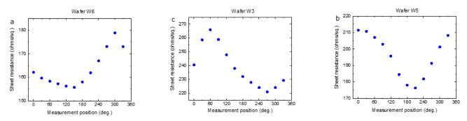
**Figure 9.** Three examples of positional variation in sheet resistance measured around the circumference of wafers 25 mm from the edge. The error bars are smaller than the symbol size.
