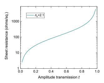
**Figure 6.** Dependence of calculated sheet resistance on the amplitude transmission *t*, assuming substrate refractive index of 2.1, as given by Equation (4).
