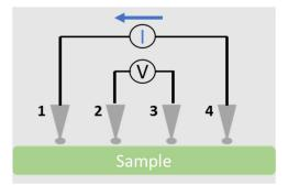
Figure 1. Schematic drawing of a four-point probe tool.
