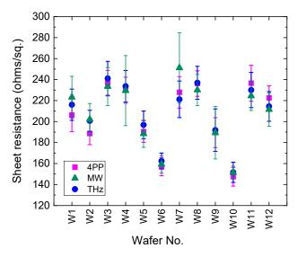
**Figure 10.** Mean sheet resistance of 12 wafers measured using the four-point probe (4pp), microwave resonator and THz time-domain spectroscopy. Each wafer was measured at multiple locations; the data points are the mean and standard deviation of all measured values.
