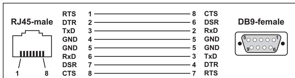
Figure 6: RJ45 to DB9 Serial Console Cable
