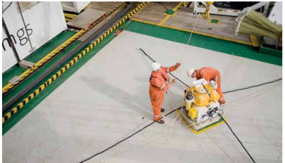
Electromagnetic receivers are placed on the seabed
