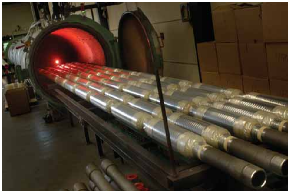
Swelable elastomer seals were invented in Shell's research lab in Rijswijk
