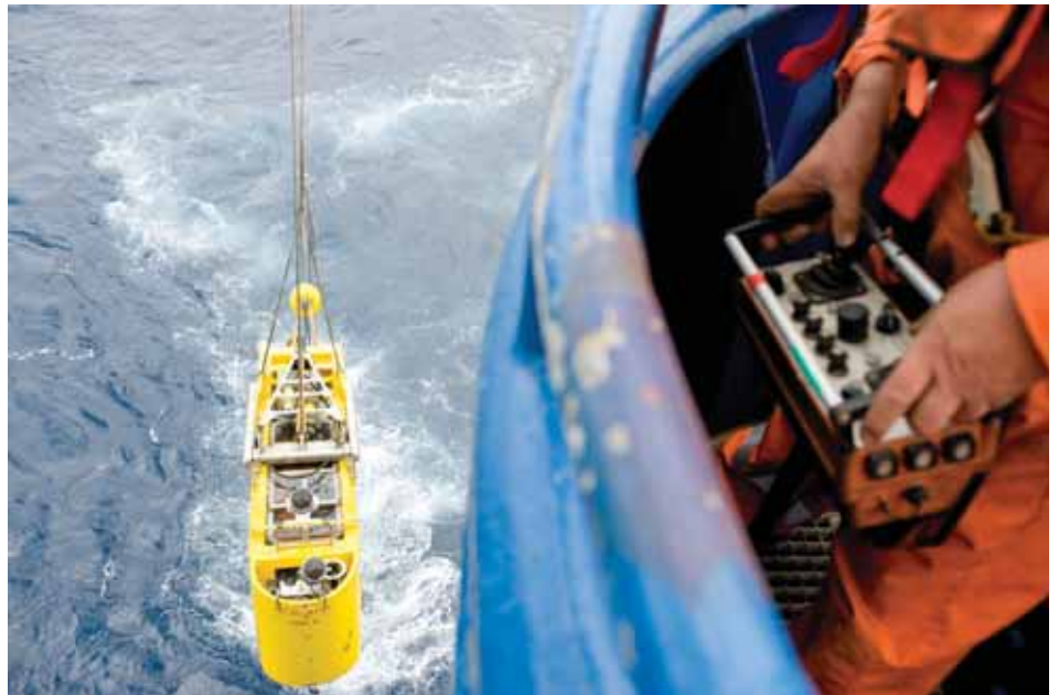
An electromagnetic source is towed from the boat
