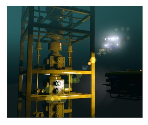
Today, the BOP Reliability Team uses the PI System to collect real-time data from all BOPs in the field. The digital BOP initiative uses available data—valve positions, wellbore pressure and temperature, alarm data, and much more—to improve BOP performance and reliability. Shell relies on custom dashboards and PI Vision to visualize the data
