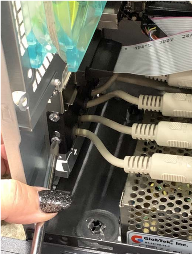
FIGURE 4—Removing the screws from the cable retaining bracket.
