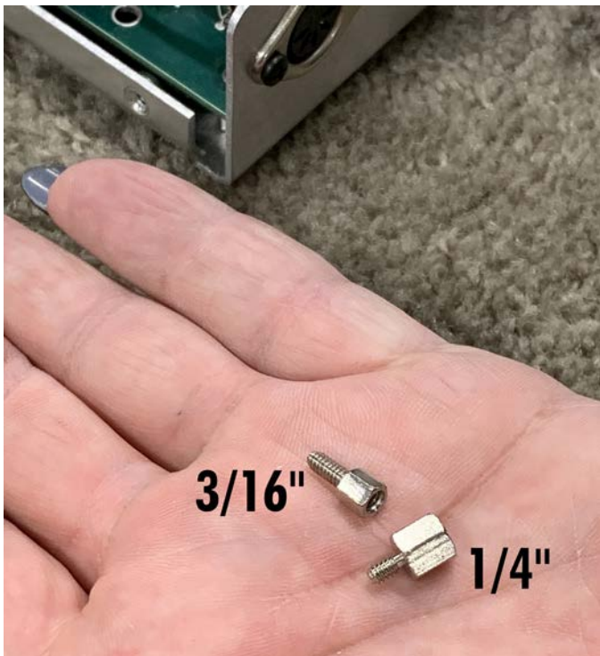
FIGURE 21—The sizes refer to the head size of the screws.
