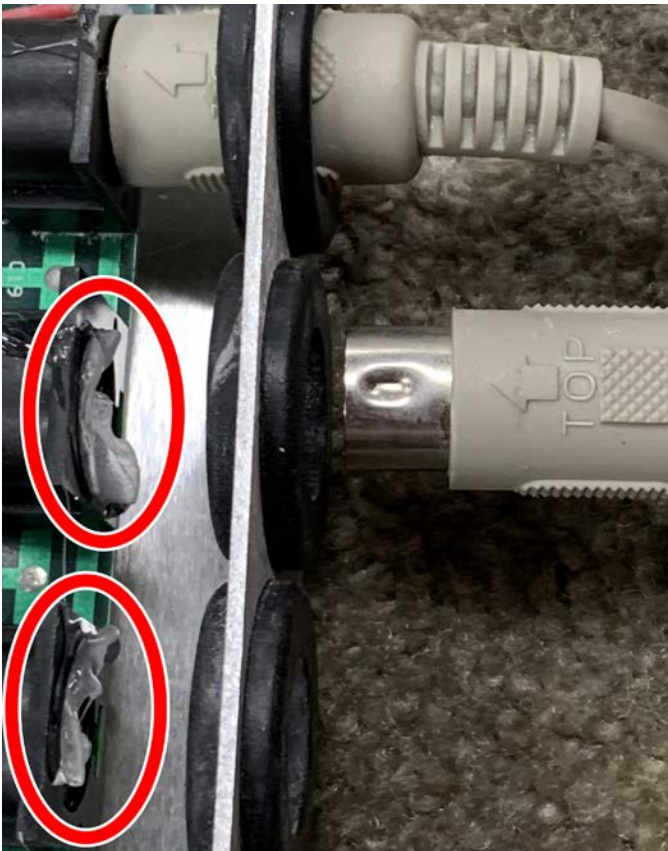
FIGURE 17—The red ellipses show the excess silicone.
