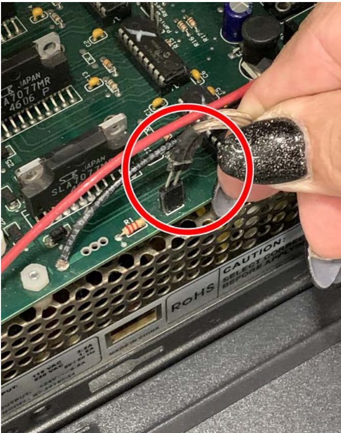
FIGURE 9—The red circle shows the location of the power light connector.
