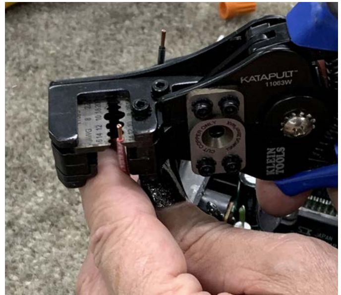
FIGURE 26—Strip off about 1/4" of the insulation.
