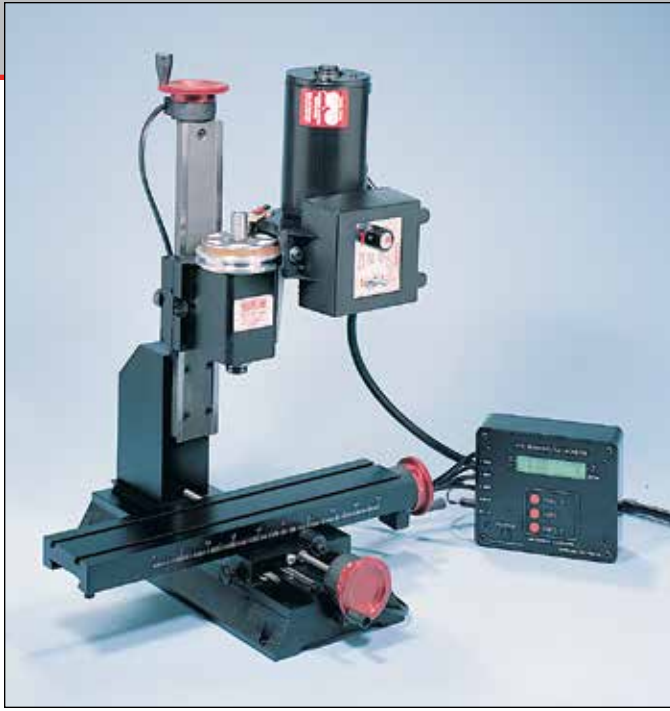
FIGURE 67—A digital readout makes life easier for the machinist. The electronic display reads out to .0005" and any axis can be reset to "zero" with the push of a button. It also helps eliminate mistakes due to losing track of the number of handwheel revolutions on longer dimensions. As a bonus, the spindle RPM is displayed at all times. The digital readout or "DRO" is available for both the lathe and mill.
