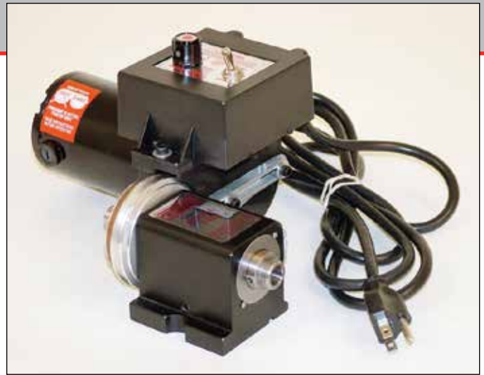
FIGURE 8—The assembled power unit.
