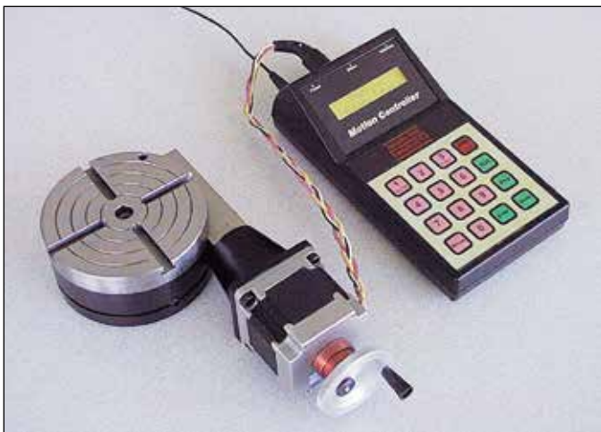
FIGURE 74—This simple programmable indexer brings computer control to operations like cutting gears.
