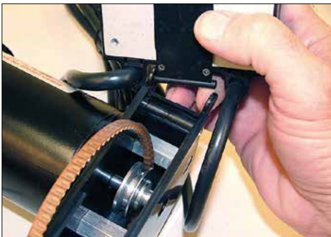
FIGURE 12—Insert "ears" of speed control housing into holes in belt guard tabs.
