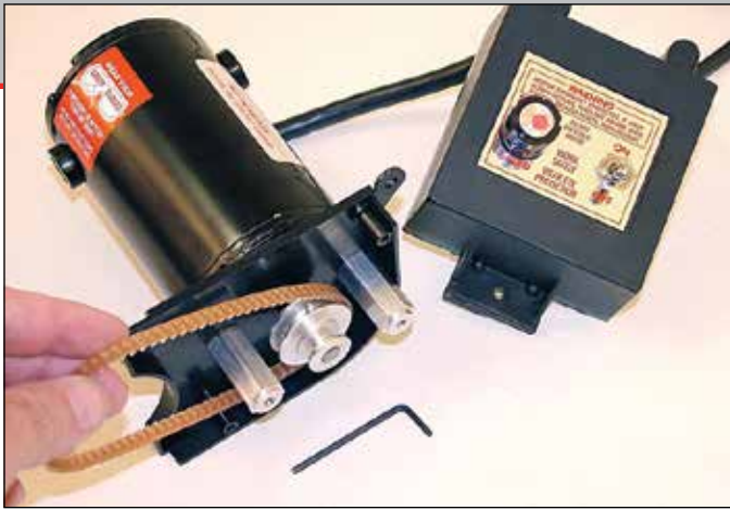
FIGURE 10—Place belt over motor pulley.
