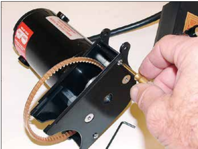
FIGURE 11—Attach outer belt guard.
