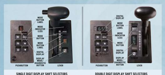
Vehicle manufacturers may choose different types of shift selectors for their vehicles. The shift selector in your Allison-equipped vehicle will be similar to one of the pushbutton or lever styles as shown above.
