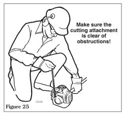
4. While holding the outer tube firmly with one hand, slowly pull the recoil starter handle until resistance is felt, then pull quickly to start the engine.
