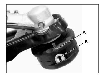
3. Insert one end of nylon line into an eyelet, and push line equal distance through trimmer head.
