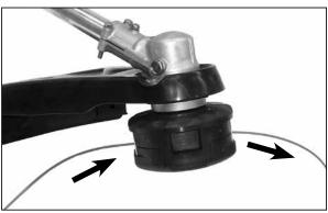
4. Hold trimmer head while turning knob (C) clockwise to wind nylon line onto spool until about 5" (13 cm) of each line remains exposed.
