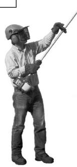
Always wear eye and hearing protection. Shindaiwa recommends wearing a face shield as additional face and eye protection.
