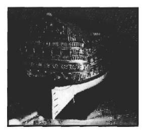
PHOTO 1. A beginner's nightmare. The stern ornamentation, the sheer of the hull, and the multiple gun decks of the San Felipe spell disaster for a first-time builder.
