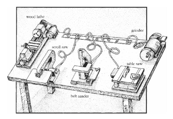
FIGURE 3 Set up a power table adjacent to your main workbench. Arrange your appliances to prevent crossed wires and awkward reaches. Most beginners won't need this much heavy artillery.
