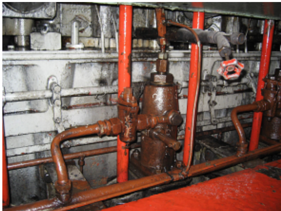
On the left: main engine oil leakages near an injection pump
