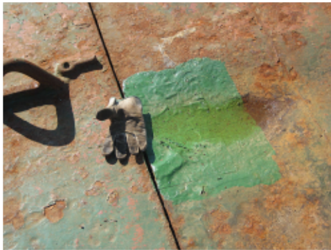
Temporary repair (tar carpet) hatchcover no. 2
