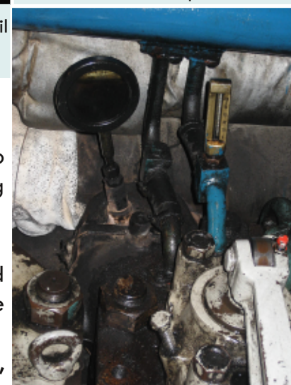
Unreadable temperature gauge in main engine cylinder no. 3
