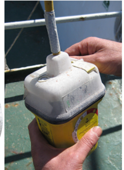
EPIRB in poor maintenance conditions and inoperative
