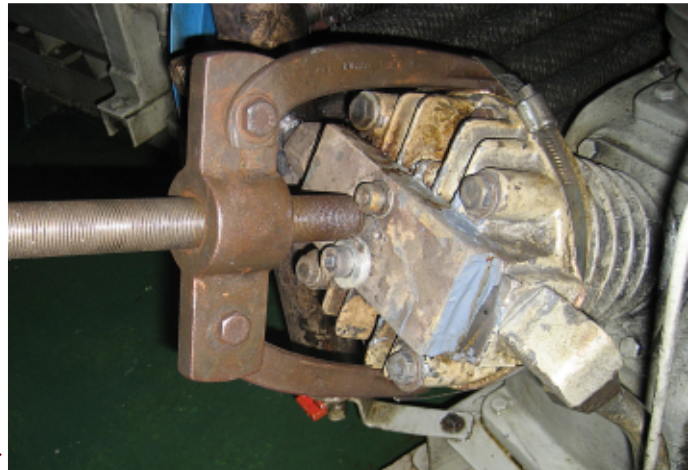
Air compressor no. 1: out of service. On the right a particular of its head temporary fixed by a gear puller
