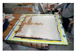
Beginning of infusion process used to wet-out the outer skin
