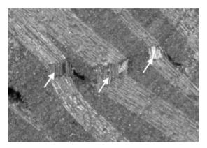
Figure 15. Formation of kink bands when composite laminates are under compression (marked with arrows) [Rakow 2006]
