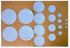
Peel ply 0.5, 1, 2, 3, and 4 inches diameter used to simulate delamination
