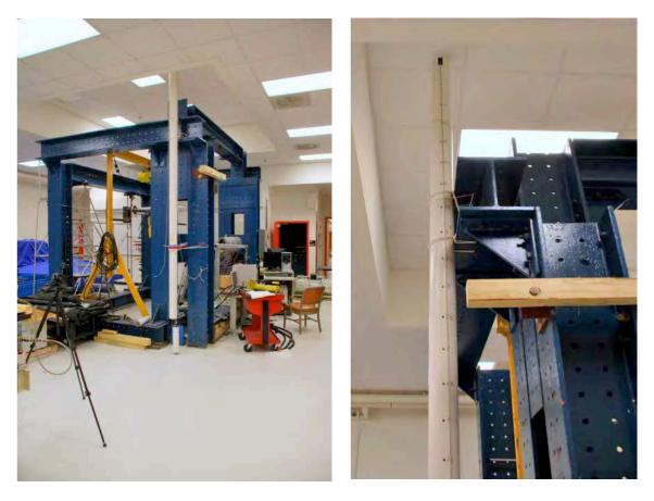
Figure 95. Impact tester at the US Naval Academy Structures Laboratory
