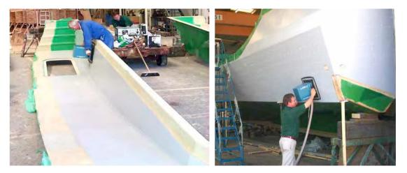
Figure 116. Vacuum hood used to test flat panel portions of RNLI lifeboat hulls [Laser Technology, Inc.]
