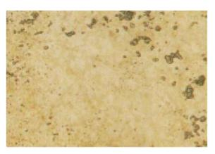
Figure 30. Image of pits or pinholes showing small regular or irregular craters on surface [Derakane 1997]
