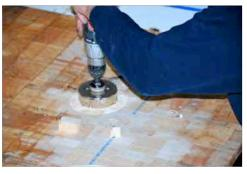
Hole saw is used to create a 1/8 inch deep void for water to be encapsulated
