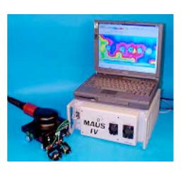
Mobile Automated Scanner (MAUS IV) UT C-scan or Low-Frequency Bond Tests (LFBT)
