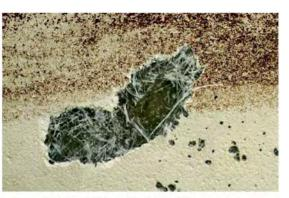
Blistering like this takes many years to develop, and will not be cured by any amount of heating or dehumidification. Peeling, blasting and thorough fresh water washing remain an essential part of the process.
