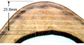
Figure 33. Composite sample close-up of apex showing extreme fiberwaviness [Anastasi 2008]
