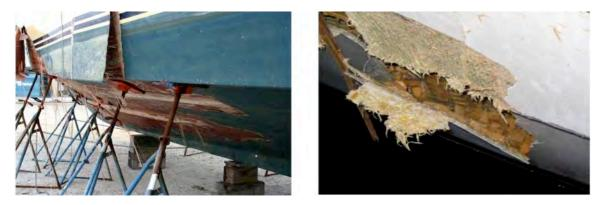
Figure 11. Examples of severe delamination resulting from manufacturing defects [www.yachtforums.com]
