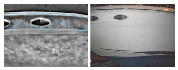
Figure 126. The dark colored anomaly noted with the blue lines is characteristic of moisture (moisture ingress was first found when the hull ports were removed). [Independent Marine Systems]
