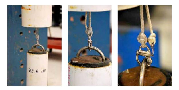
Figure 94. Detail of impactor release mechanism
