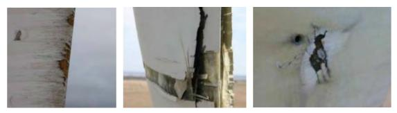
Figure 73. Wind blade damage showing: Leading Edge Erosion, Severe Blade Damage (left) , Delamination (center) and Lightning Damage to Blade [Knight & Carver]
