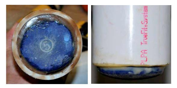
Figure 93. Rubber coated barbell is epoxied into PVC tube to form impactor
