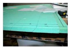
45° saw cuts (3, 6 and 12 inches long) in core used to simulate core shear failure
