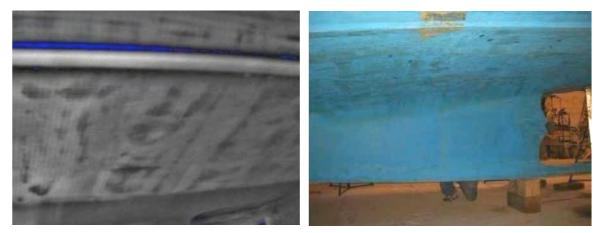
Figure 125. This vessel had anomalies on the entire port side of the hull bottom that were characteristic of moisture ingress. Two hole saw samples were taken and both sampled areas produced water when drilled into. [Independent Marine Systems]
