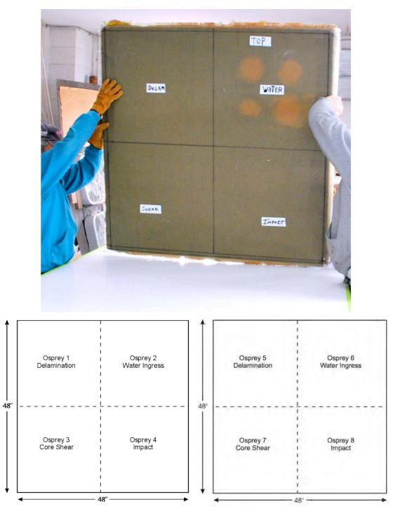
Figure 86. Layout of E-glass @ 3.29 lbs/ft<sup>2</sup> test panel (left) and carbon fiber panel @ 2.16 lbs/ft<sup>2</sup> (right). Note in photograph that the area where water ingress was simulated is clearly visible before being covered.
