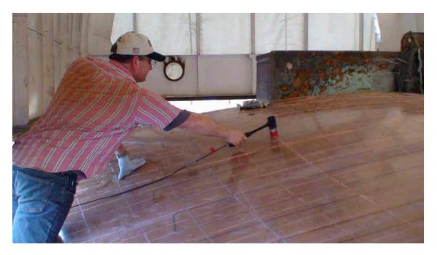
Figure 55. An instrumented hammer is used to excite a composite destroyer rudder during SIDER examination [author photo]
