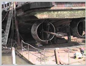
Kort nozzles are engineered to improve the flow around the propellers. They are similar in some ways to an airplane propeller. The propeller shaft on this vessel is being 'pulled'. Propulsion systems on vessels are inspected and worn parts are replaced at each drydock opportunity.
