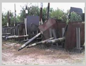
ome vessel operators have spare rudders built and in storage at a shipyard so they will be ready on short notice.
