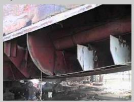
**Frames** in the **void** wing tank of a river barge. In this photo, the knuckle plate has been cut away so that bent frames can be renewed. The **double bottom** is exposed. New knuckle plate will be installed once the frames are renewed.
