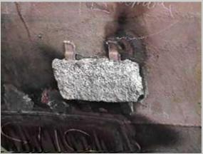
This anode has been partly sacrificed by electrolysis on this vessel. It is still in good enough shape to keep on the vessel and is doing its intended job very well.
