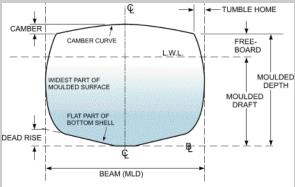
Fig. 3 Moulded Dimensions of Midship Section
