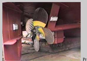
opeller on a river towboat. This one has 4 blades and is designed for power rather than speed. 4 blade propellers have less vibration than 2 or 3 blade propellers, benefiting the crew.
