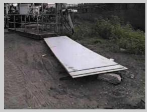
A stack of plates that will be used for side shell replacement, frames, brackets, etc.... These plates have been sandblasted and coated to reduce corrosion inside the vessel once they are installed.
