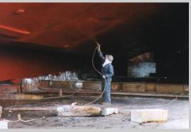
ainter applying a coating to a vessel hull.
