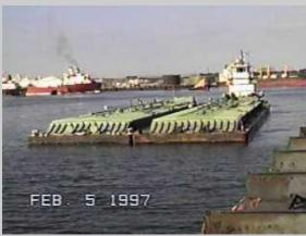
These 2 **tank barges** are loaded with petrochemicals in the Houston, Texas, USA ship channel. The boat that is pushing them is called a **tow boat**, because it pushes a 'tow of barges'.
