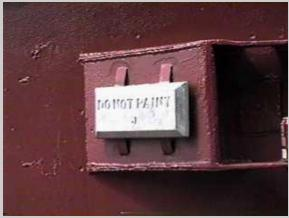
This is a new anode on a vessel, it has been welded in place. The shipyard did a good job of not painting the anode.
