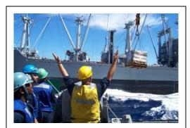
Fig. 2-22. Ship-to-ship onloading
