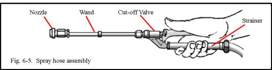
The cutoff valve or trigger assembly is a spring-loaded valve to regulate the spray flow rate. Poor-quality or poorly-maintained cutoff valves do not completely stop the pressurized flow of liquid, resulting in some pesticide dripping from the nozzle.
