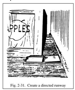
• The conventional wood base, spring (snap) trap is also an effective way to kill rats and mice. Set traps at right angles to the runway, with the trigger end toward the bulkhead. Once traps are in use, replace bait every 2 days. On the deck, set traps behind objects that are stacked close to a bulkhead, along rows of boxes and between crates. Boxes and barrels can be positioned to create directed runways to force the rodents to pass over the traps (Fig. 2-31).
