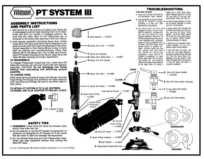
Fig. 6-1. Whitmire® PT® System III aerosol container pesticide dispersal unit.
