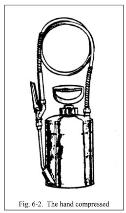
high reliability. The hand-compressed sprayer ranges in size from a one-half to two-gallon cylindrical tank, fitted with an air pump, hose, spray gun, and other components necessary for applying liquid insecticide formulations.
