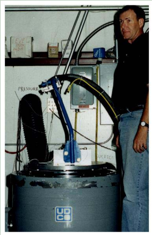
Electro-magnetic shaker with 15000 pounds of force
