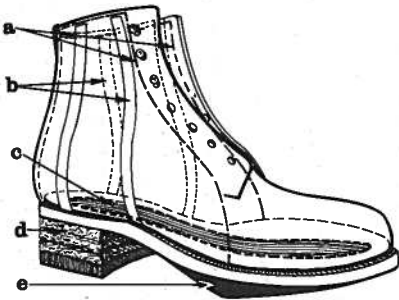
FIGURE 29. High-quarter shoe with combination of modifications prescribed for a painfully ankylosed ankle or foot. (a) High bilaterally extended counter; (b) reinforcing steels; (c) long steel spring; (d) SACH heel; (e) rocker bar. If the patient were obese, medial and lateral shank fillers would be used, and the SACH heel replaced by a heel of regular hardness to prevent rolling or vaulting over the shank fillers from heel strike to toe-off.
