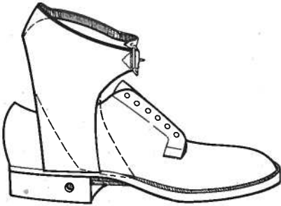
FIGURE 16. Valgus corrective strap; dotted line indicates more effective placement. (Note hole in heel for caliper-box attachment.)
