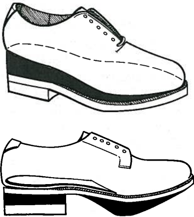
FIGURE 28. Heel elevations. Top: sandwich; bottom: combination insert-sandwich division with rocker bar installed as integral part of cork elevation to facilitate faster rollover.
