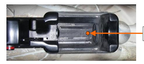
Check that any screws do not protrude into receiver
