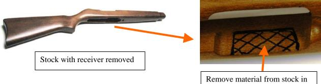
Remove material from stock in this area on both sides
