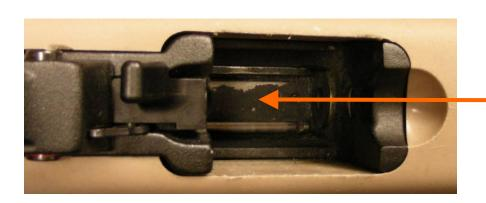
Check for and remove any large amounts of paint in this area.
