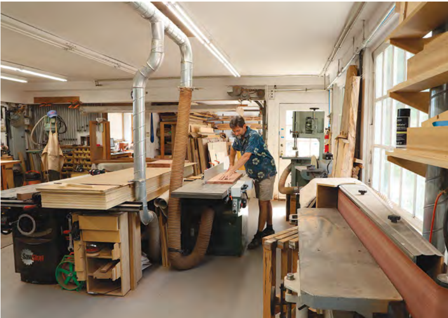
An island for organization. To make the most efficient use of his 800-sq.-ft. machine and bench space, Throop located his SawStop tablesaw and Felder jointer/planer side by side as an island in the middle with walking space around them and arrayed his other machines along the walls.
