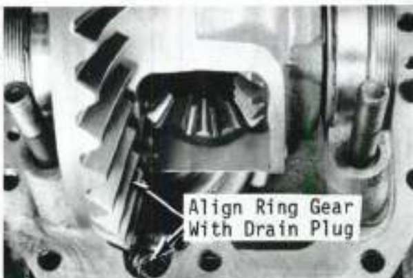
Fig. 36—When installing differential unit in carrier housing, make certain ring gear is on same side as housing drain plug.
