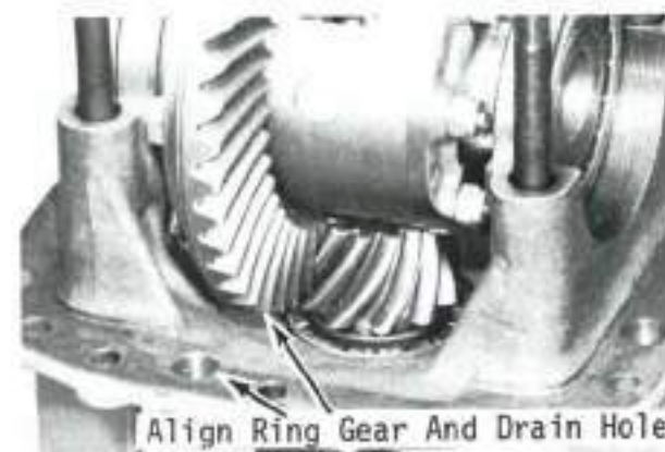
Fig. 29—When installing differential unit in carrier, make sure ring gear is on same side as drain hole in carrier.
