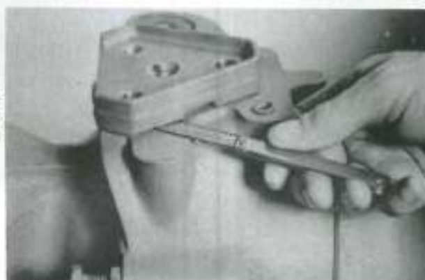
Fig. 33—To set swivel bearing preload, measure gap between swivel pin and swivel housing with a feeler gauge. Refer to text.
