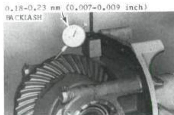
Fig. 15—View showing proper placement of dial indicator for setting backlash in front drive differentials.
