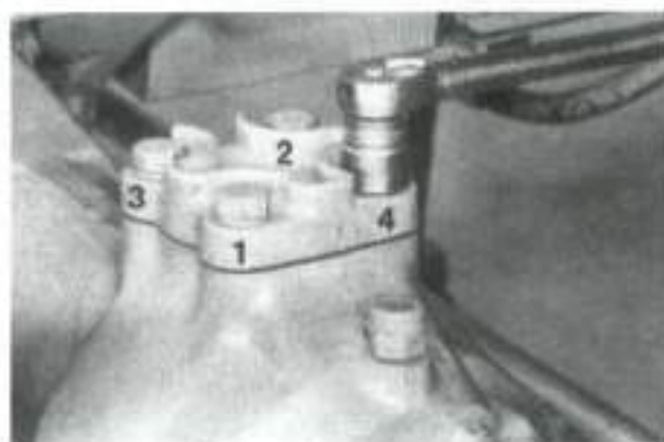
Fig. 22—Proper tightening sequence used to install bearing pin cover prior to setting bearing pin preload.
