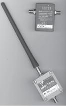
cepts 11-15 VDC through a 5.5/2.1mm jack or via a 5V USB B port. The power then travels up the coax cable to power the antenna. The inserter features a BNC antenna jack for coax from the antenna element and a BNC jack output to the receiver. This flexibility makes it well suited for portable use. Made in Germany.
