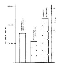
Fig. 28 Effect of Peening and Scratches on Endurance Limit of 4340 Steel at Rc51
