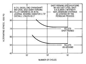
Fig. 30 Increase in Fatigue Strength of Shot Peened Crankshaft
