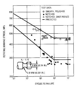
Fig. 36 Fatigue Tests on Notched Shafts
