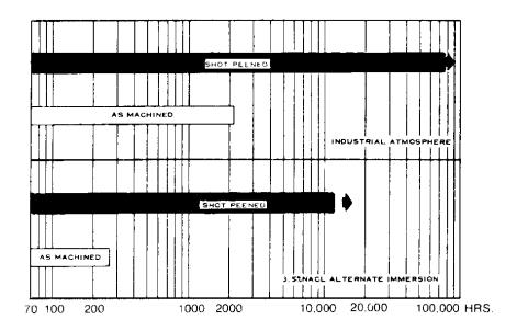
Fig, 25 Effect of Peening on Resistance to Stress Corrosion Cracking of 7075-T6
