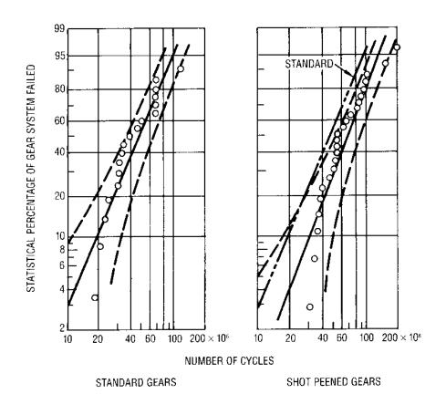
Fig. 23 Comparison of Surface (Pitting) Fatigue Lives of Standard Ground and Shot-Peened Carburized and Hardened CVM AISI9310 Steel Spur Gears, Speed, 10,000 RPM; Lubricant, Synthetic Paraffinic Oil; Gear Temp. 350K (170 f) Maximum Hertz Stress, 1.7X10 N/m (248,000 psi)
