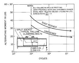
Fig. 21 L-N Curve Clamped Up Joint 4140 Steel
