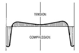
Fig. 3 Typical Residual Stress Distribution After Peening
