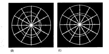
FIG. 46 Contour Correction of Ring Gear (B) Before Peen Forming (C) After Peen Forming
