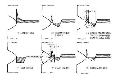
Fig. 24 Crack Arrest by Compressive Self Stress
