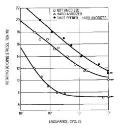
Fig. 14 R.R.Moore Fatigue Strength of Titanium 6AL-4V Polished vs. AS - Sprayed Coating with Pre-spray Conditioning Grit Blast and/or Shot-Peen - METCO 64F
