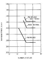
Figure 16 Effect of Shot Peening on Welded STE690 Material
