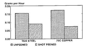
Fig. 19 Rate of Material Loss by Cavitation
