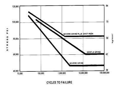
Fig. 7 Reversed Bending Fatigue of Flat Bars of Rockwell Hardness C45
