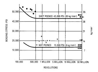
Fig. 35 Fatigue Tests on Rear-axle Shafts
