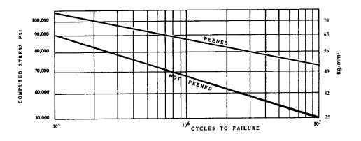
Fig. 34 Fatigue of Carburized Gears
