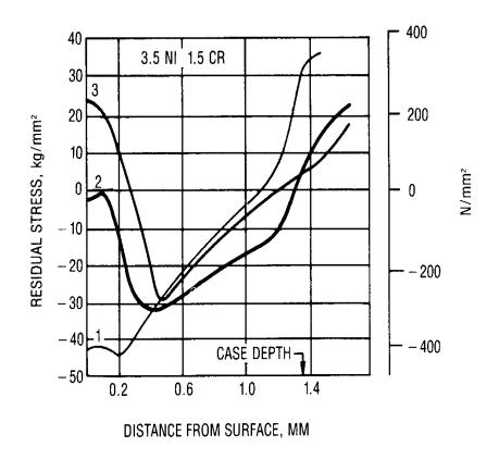
Fig. 18 The Effect of Decarburization on the Residual Stresses Developed in Carburized and Hardened Plates. The Carbon Content at 0.002mm Was Estimated to Be: CURVE 1, 1%; CURVE 2, 0.64%; CURVE 3, 0.35%
