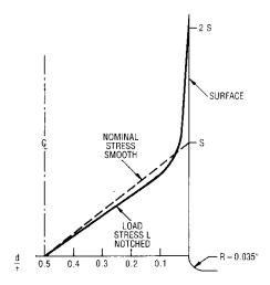
Fig. 5 Distribution of Bending Stress in a Notched Beam
