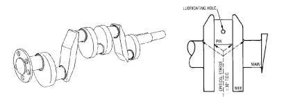
Fig. 31 Crankshaft and Detail
