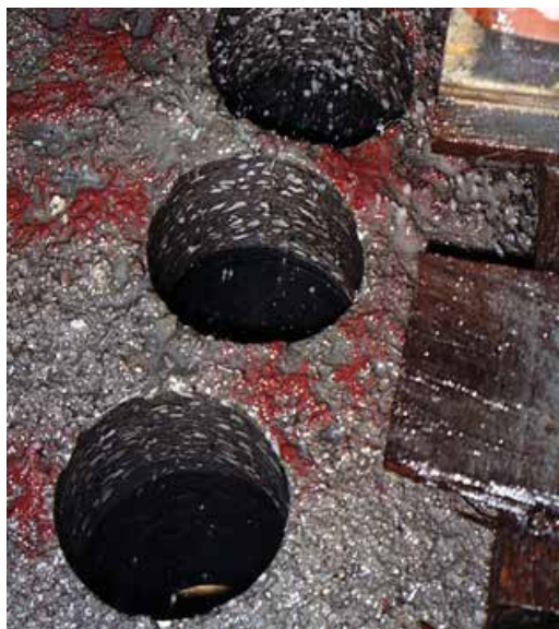
Fig. 3: Coring of a test panel
