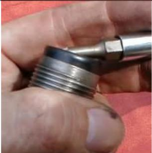
Remove the spring, plug, and follower toward the front. Removal of the magazine cutoff spring screw will have freed the magazine tube, and it can be unscrewed from the receiver. (It is not recommended that you remove the magazine tube for normal takedown but can be removed if repair is necessary. The tube is very tightly screwed into place and will require effort to remove.
