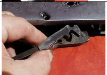
3. When installing the combination trigger and safety detent spring. Use a tool to depress the spring at the cross pin location. And insert a small punch to hold the spring down while putting in the cross pin. It will be necessary to depress the spring on the other side as the pin is inserted, and the end of the cross pin must also be depressed as it enters the hole on the other side of the tang.
