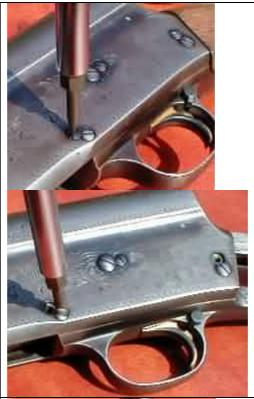
8. Remove the lock screw, then the main screw on the left at the lower rear of the receiver.
