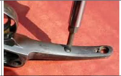
14. Insert a small screwdriver at the front of the safety sear to depress the plunger and spring, and remove the safety sear toward the left. (Remember the spring and plunger are under pressure, keep them under control as you remove the safety sear) then remove the plunger and spring upward.
