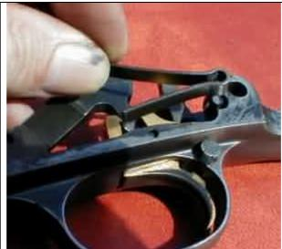
11.Move the safety to the off-safe position, tip the safety sear forward, restrain the hammer, pull the trigger, and ease the hammer forward until its roller disengages from the tip of the hammer spring.
