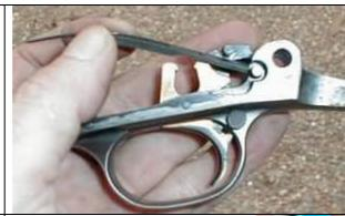
16. Push out the small cross pin in the rear of the trigger housing, Removal is easier if he trigger spring is slightly depressed in the vicinity of the pin. (Note: Newer model have a slots cut on each side of the inter part of the spring recess. There are tabs on both sides of the safety spring that slide up and into the slots)
