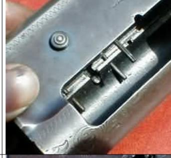
2. In the later guns that have the two piece carrier, the arrangement of the parts may be difficult for the novice. In this picture, the parts are shown in the proper position. Hold to gather and insert them in the bottom of the receiver aligning the holes on the side of the receiver with the holes in the carrier sides. Insert both carrier screws before you release the carrier.
