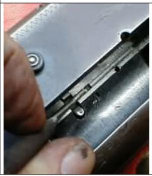
And this one shows all the pin in an exaggerated state so you can see where they come out and not let them go too far into this slide area as you reinstall. (note: this is also the direction they are removed.
