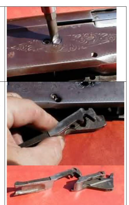
22. Remove the two sections of the carrier downward. Note that on earlier guns, the carrier will be a single part. Later models are a two-part system.
