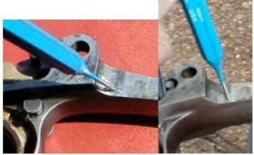
17. Remove the trigger spring upward and toward the rear. Or slide it out if it has rails cut into the receiver.
