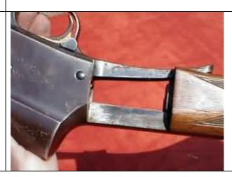
7. Remove the lock screw, then the main screw on the left side of the receiver, just above the front trigger housing.
