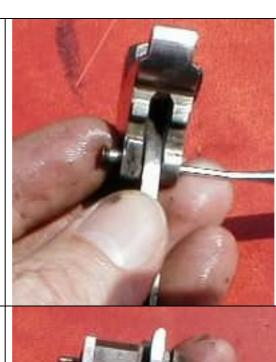
32. The extractors and their coil springs are retained on each side at the front of the bolt by vertical pins. Punch out the pins downward, and take the extractors and springs out toward each side.
