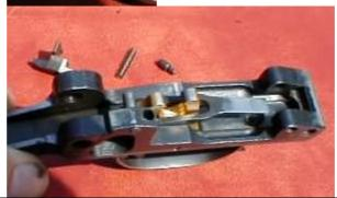
15. Lift the hammer spring at the front, and remove it upward and toward the front.
