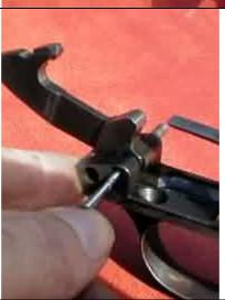
13. Remove the hammer spring screw, located on the underside of the rear tang of the trigger housing. (Note: that the spring is not removed at this time).
