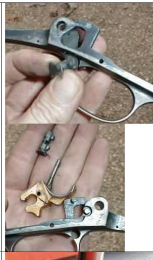
21. Remove the lock screw and the large carrier pivot screw on each side of the receiver.
