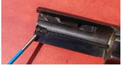
3.Remove the bronze friction piece and it's attached spring toward the front. Note that this picture shows the rings in a normal setup for high to magnum loads.
