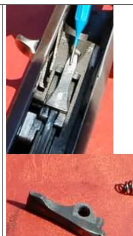
27. Move the bolt to the rear, swing the link bar outward. Restrain the operating handle, and move the bolt forward, leaving the handle at the rear.
