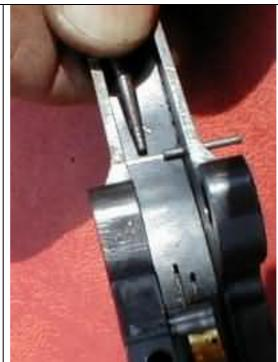
4. When installing the trigger group in the receiver. Insert the front first. You will need to hold pressure to keep it in line with the front hole. Once you have the front pin in place but not screwed you can pull the action handle back about one inch and the rear of the trigger guard will go in place. Make sure that the carrier spring is riding on the carrier dog as you are attempting to put the front of the trigger guard in place.
