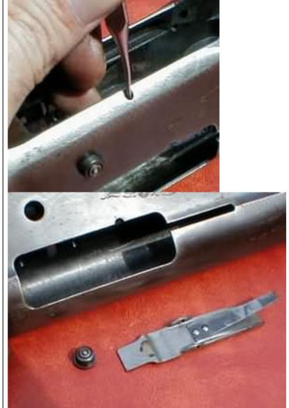
38. Insert a screw driver in the opening center of the magazine spring retainer, and pry the retainer out, moving the screwdriver to raise the retainer equally around the edge until it is loose enough to remove. **Remember:** The magazine spring is under tension, be sure to control the retainer and ease it out until the tension is removed.
