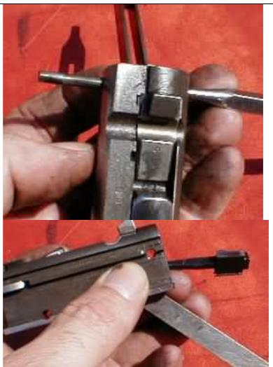
31. Push the front of the link bar upward, tipping the locking block out the top of the bolt, and remove the assembly upward. Punch out the cross pin at the lower rear of the locking block and it will release the link bar for removal.
