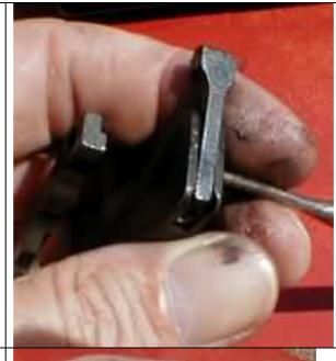
24. Restrain the bolt spring plug at the rear of it's housing, push out the cross pin, and remove the plug, spring, and follower toward the rear. (Note: The spring is very strong, and is under great tension. Make sure to control it and ease it out) It is also possible to unscrew the housing (tube) from the rear tang of the receiver on older models, Newer models are soldered into place). I would not remove those that screw in during normal cleaning breakdowns only for repair.
