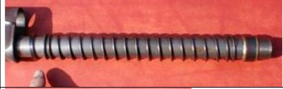
This next picture shows the rings bevel and flat side. Note when the ring is on the bottom close to the receiver the bevel goes toward the receiver and when on top the flat side goes toward the spring.
