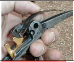
18. Invert the trigger housing over the palm of the hand, and move the safety to free the detent ball. If it does not drop out easily, tap the housing with a nylon or wood hammer.
