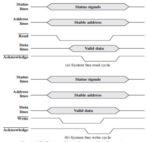
Figure 1.21 Timing of Asynchronous Bus Operations
