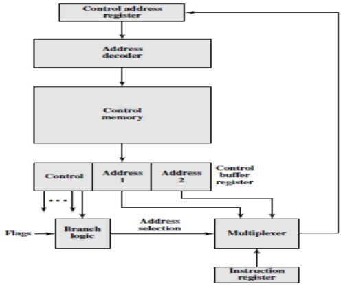
Figure 5.5 Branch Control Logic: Two Address Field
