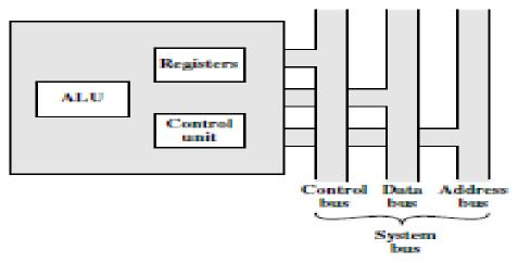
Figure 2.6 The CPU With System Bus
