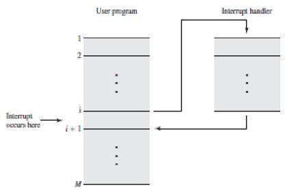
Figure 1.10 Transfer of Control via Interrupts
