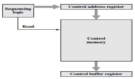
Figure 5.3 Control Unit MicroArchitecture
