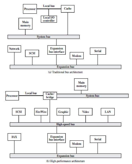
Figure 1.19 Example Bus Confiburation
