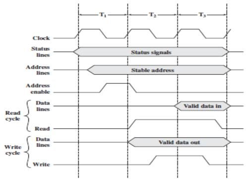
Figure 1.20 Timing of Synchronous Bus Operations
