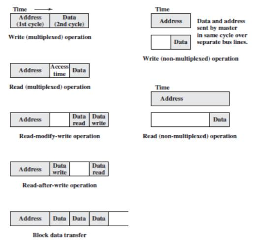
Figure 1.22 Bus Data Transfer Types
