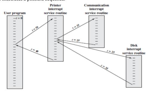
Figure 1.16 Example Time Sequence of Multiple Interrupts
