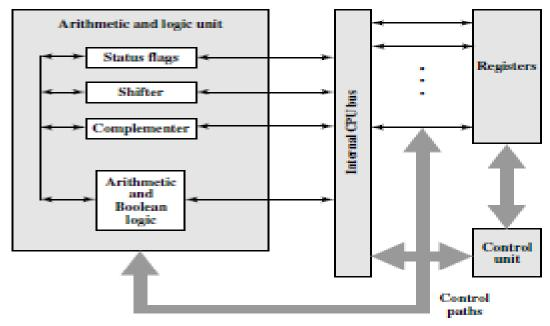
2.7Internal Structure of the CPU
