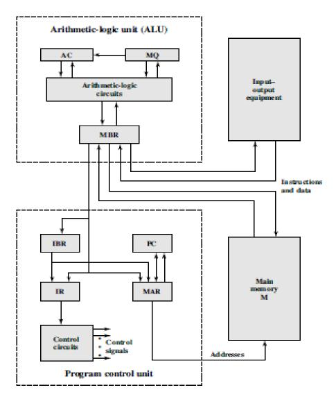
Figure 1.2 Expanded Structure of IAS Computer
