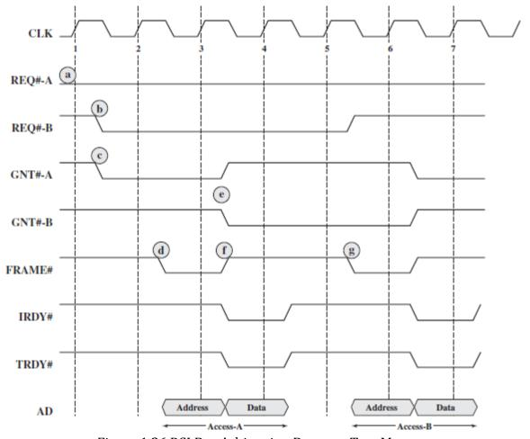
Figure 1.26 PCI Bus Arbitration Between Two Masters
