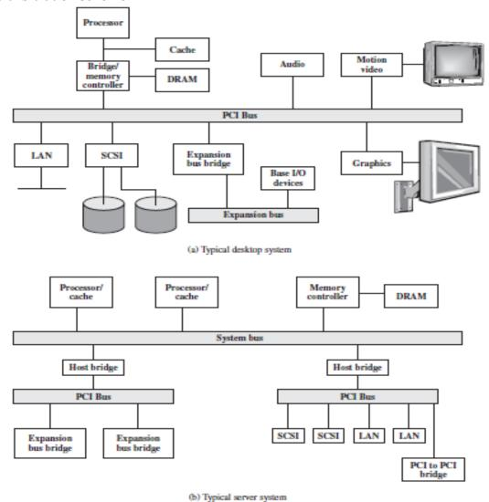
Figure 1.23 Example PCI Configurations
