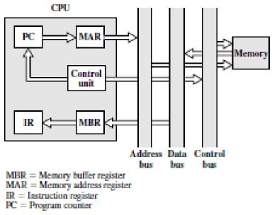
Figure 2.11 Data Flow, Fetch cycle
