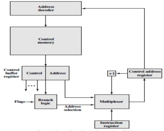
Figure 5.6 Branch Control Logic: Single Address Field
