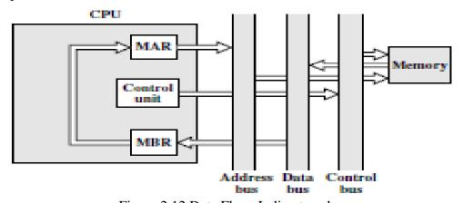
Figure 2.12 Data Flow, Indirect cycle
