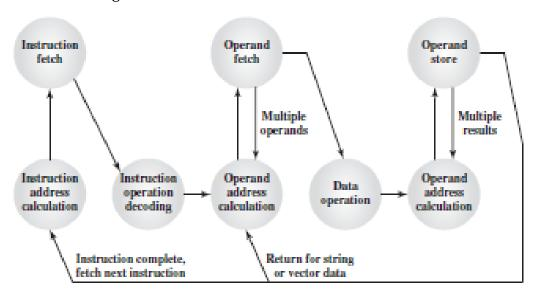
Figure 1.8 Instruction Cycle State Diagram
