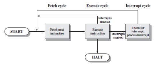
Figure 1.11Instruction Cycle with Interrupts
