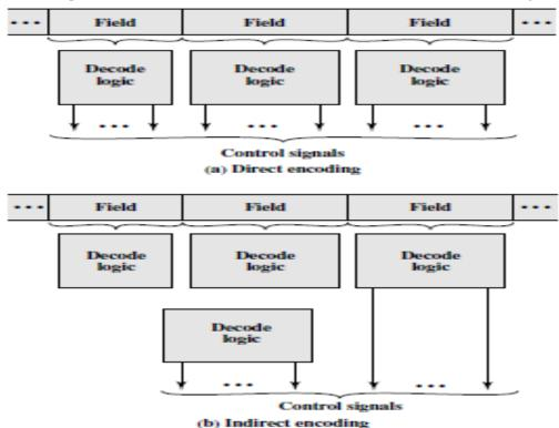
Figure 5.8 MicroInstruction Encoding
