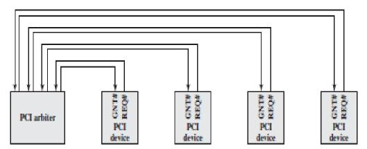
Figure 1.25 PCI Bus Arbiter
