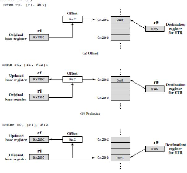
Figure 2.3 ARM Indexing Methods
