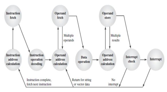
Figure 1.14 Instruction Cycle State Diagram With Interrupts
