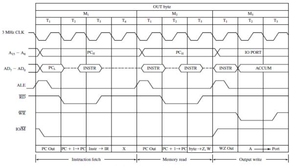
Figure 4.7 Timing Diagram for Intel 8085 OUT Instruction
