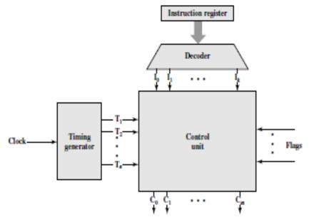
Figure 4.8 Control Unit with Decoded Inputs
