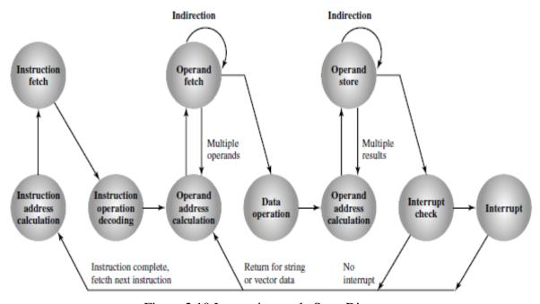
Figure 2.10 Instruction cycle State Diagram
