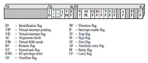
Figure 3.9 PentiumII EFLAGS Register
