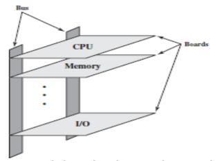
Figure 1.18 Typical Physical Realization of a Bus Architecture
