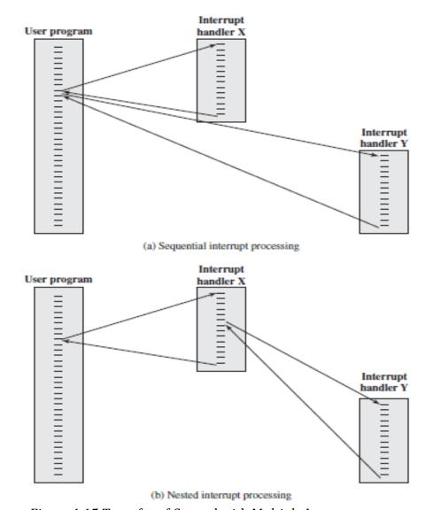
Figure 1.15 Transfer of Control with Multiple Interrupts
