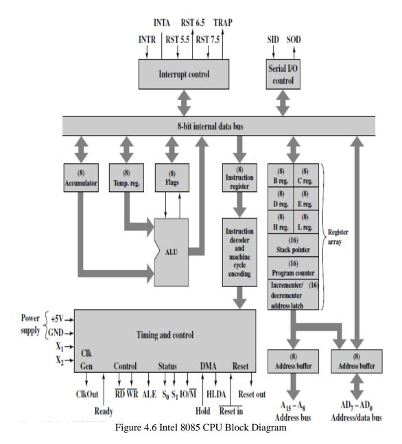
Table 4.2 describes the external signals into and out of the 8085. These are linked to the external system bus. These signals are the interface between the 8085 processor and the rest of the system.
