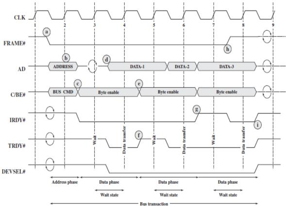
Figure 1.24 PCI Read Operation
