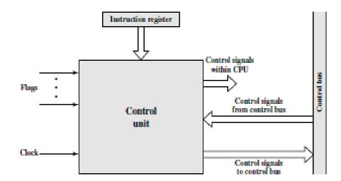
Figure 4.4 Block Diagram of Control Unit
