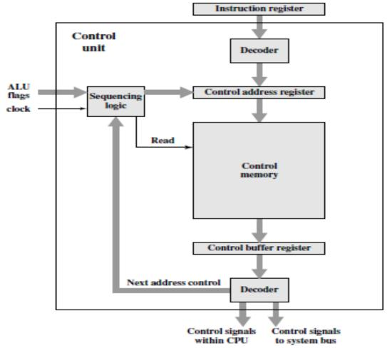
Figure 5.4 Functioning of microprogrammed control unit
